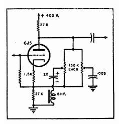
Fig. 17-22. Single-ended tone control circuit.
