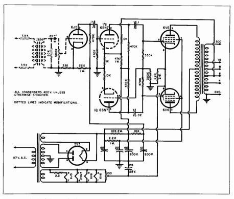
Fig. 26-2. Schematic diagram of the monitor amplifier using conventional circuits.
