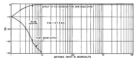
Fig. 24-11. FM limiting characteristics.
