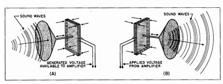
Fig. 4-24. (A) Microphone (generator) and (B) headphone (motor) action.
