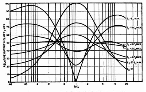
Fig. 19-24. Frequency response for circuit of Fig. 19-19 for different settings of R1.
