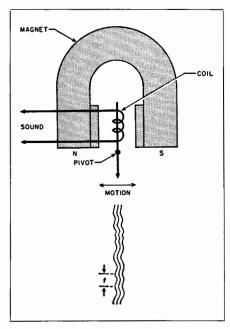
Fig. 3-1. Simplified construction of the electromagnetic cutter and its actian.
