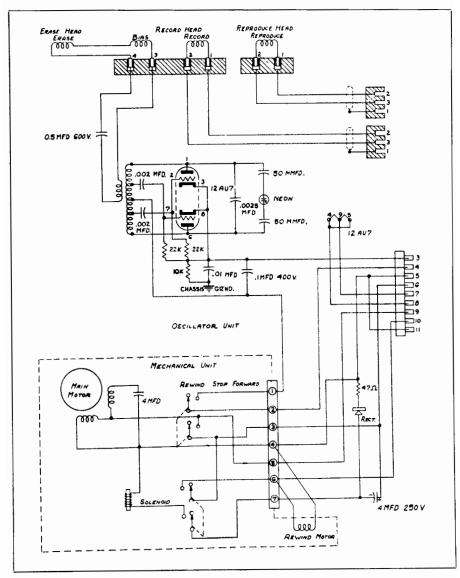
Fig. 12-36. Schematic of the Magnecorder PT63-A Oscillator Unit.
