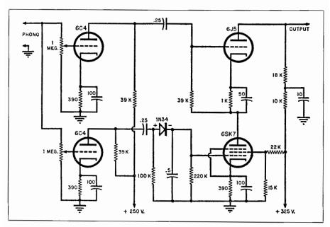
Fig. 19-44. Typical voltage amplifier circuit, incorporating the expander.
