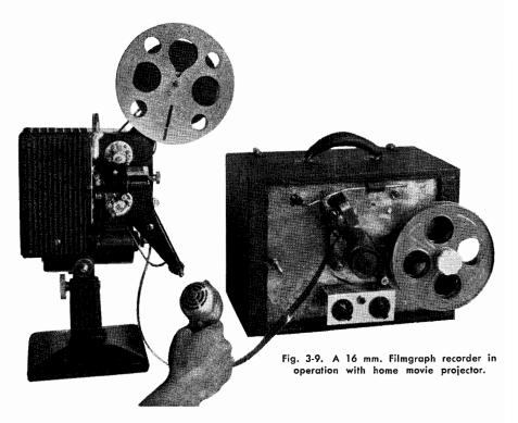
cal sound track, however, is so satisfactory for most sound on film work that it has been used almost exclusively. Magnetic recording of motion picture film offers some real advantages over other systems and is rapidly taking its place with accepted techniques.
