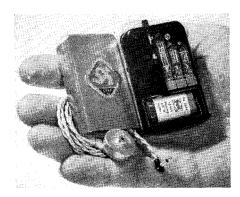
Fig. 12-33. Madel AP-8 Miniaturized Playback Amplifier. (Courtesy Stancil-Hoffman Corparation)
