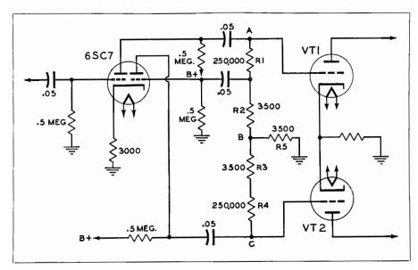
Fig. 19-14. Modified arrangement af Fig. 19-12. This circuit compensates for part of the unbalance that might otherwise accur.
