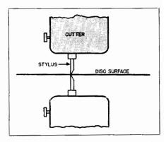
Fig. 7-6. Correct cutting angle of a stylus may be checked by viewing the reflection of the cutting stylus on the shiny surface of an uncut blonk when the turntable is in a stationary state.
