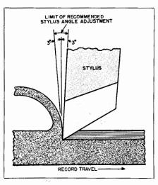
Fig. 7-1. Stylus angle adjustment.
