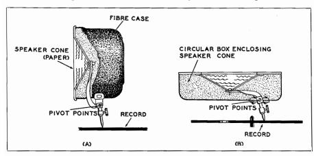
Fig. 2-4. Two relatively new types of acoustical sound reproducers.
