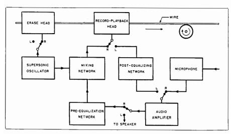
Fig. 11-6. Simplified block diagram of a typical wire recorder.
