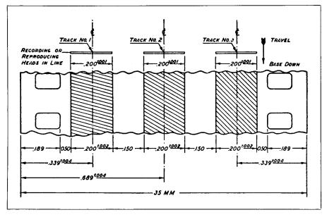
Fig. 13-1. Proposed mognetic film-track standards.
