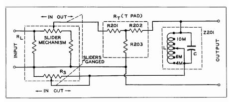
Fig. 18-3C. Simplified diagram of the Presto automatic equalizer.
