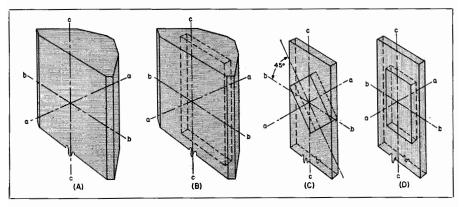
Fig. 4-25. Illustrating how crystals are cut to form "bender" and "twister" elements.
