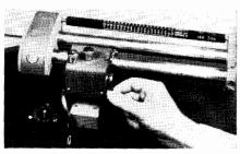
Fig. 5-24. Cutter-head is raised or lowered by this lever and permits gentle action.
