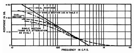
Fig. 20-6. Comparison of response curves for flat, 500 cps equalizer shown in Table 1B.
