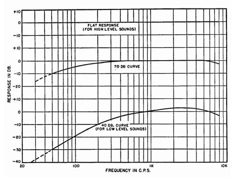
Fig. 23-8. Frequency response characteristics recommended as stondard curves for noise level measurements.
