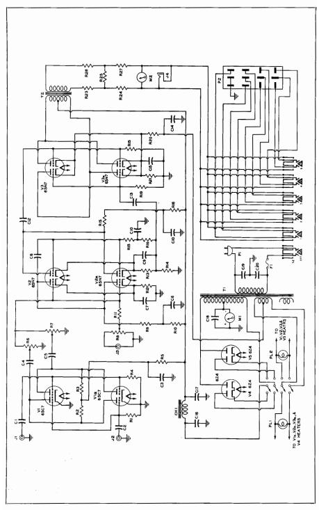
Fig. 19-25. Complete circuit diagram of amplifier.
