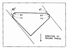
Fig. 7-14. Cross-section of same Anti-Noise Modulation Stylus in a groove whose slope is 40°. Leading facet 2b functions at an angle of 5° on the side where groove slope diminishes the burnishing angle. Facet 1a burnishes the opposite wall at 55°. (Courtesy, F. L. Capps)
