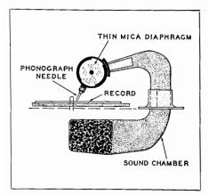
Fig. 2-3. Old type mechanical reproducer.
