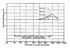
Fig. 13-8. Recording-amplifier gain-frequency characteristics.
