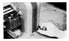
Fig. 5-26. Adjustment of pitch is made by this conveniently located control knob. (Courtesy, RCA)
