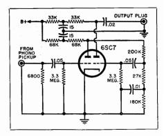
Fig. 9-18. Preamplifier and equalizing circuit used in conjunction with the General Electric variable reluctance pickup. Like extremely high fidelity microphones, this reproducer's autput voltage is low.
