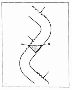
Fig. 7-12B. Diagram of a highly modulated groove showing areas (arraws) which will be rough where the burnishing facets (1a and 1b) cannot function properly. (Courtesy, F. L. Capps)
