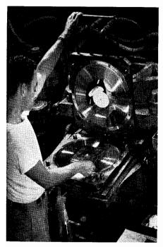
Fig. 27-14. The heat and high pressure of the stamping machine form the transcription from either special plastic or shellac material.
