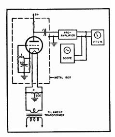
Fig. 28-28. Setup for measuring tube hum.
