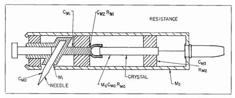
Fig. 9-26. Construction of the Bimorph type phono cartridge.
