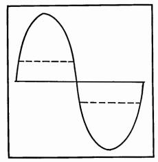
Fig. 28-18. Principle of clipper circuit. Peaks of sine wave are clipped to get square wave.
