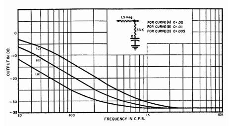
Fig. 20-2. (A) Equalizer for flat recordings with 250 cps turnover. (B) Equalizer for flat recordings with 500 cps turnover. (C) Unit for flat recordings with 1000 cps turnover.
