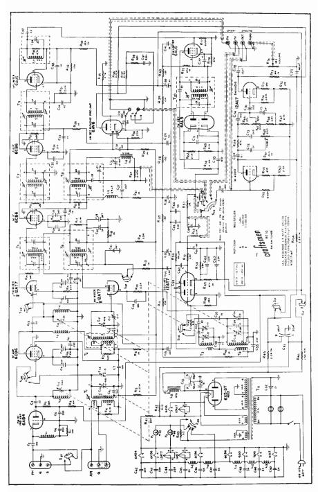
Fig. 24-10. Complete schematic of the RC-10 AM-FM tuner preomp.
