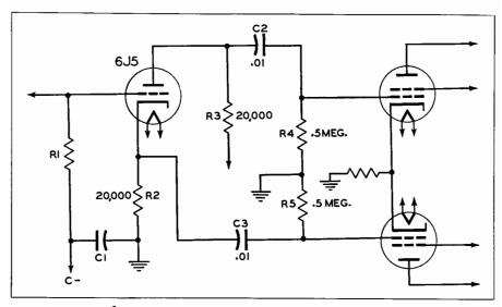
Fig. 19-10. The 180° phase shift, necessary for proper phase inversion, is obtained by taking advantage of the signal voltage on the cathode of the 6J5 triode tube.
