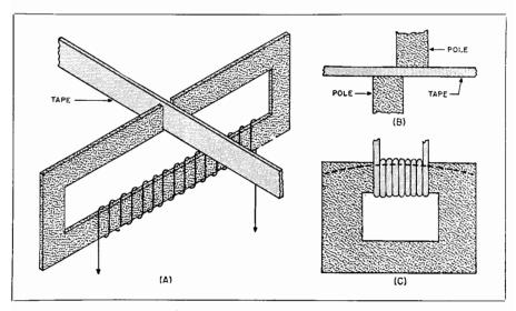
Fig. 3-21. Simplified diagrams of (A) record-reproduce head for transverse recording on tape, (B) offset, thick pole pieces which improve characteristics of head shown in (A), and (C) closed type wire record-reproduce head.
