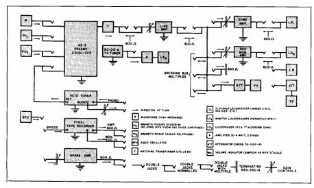
Fig. 26-8. Block diagram of the complete recording system using components discussed in the text.
