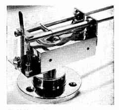
Fif. 10-12. Detailed construction of the Goodell Duplex reproducer orm.
