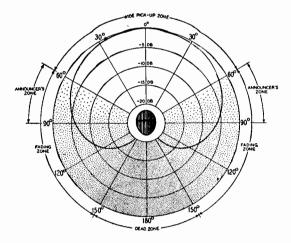
Fig. 14-17. Reference chart far interpreting the performance of the 639A microphone.
