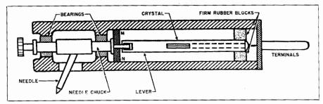
Fig. 9-8. Motions of the needle chuck ore transmitted to the crystal via lever action in this Shure-designed crystal cartridge.
