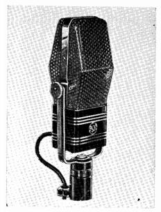
Fig. 14-11. The velocity microphone which is also known as a "ribbon type."
