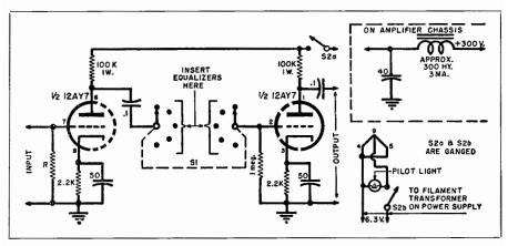
Fig. 20-5. Circuit diagram of preamplifier. Equalizers connect to Switch S<sub>1</sub>.
