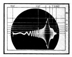
Fig. 28-10A. Unretouched oscillogroph of the response of the No. 253 offset stylus when used with the RV 20 1 pickup. No equalization. (This oscillogram was taken using the Clarkstan No. 1000A Audio Sweep Frequency Record.)
