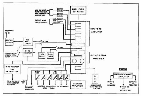
Fig. 22-12. Block diagrom of instantaneous switching panel and associated truck equipment.
