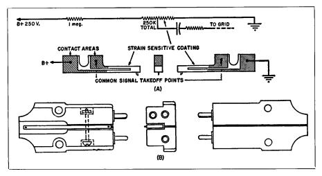
Fig. 9-10. (A) Active elements with integral stylus. (B) Cartridge with strain-sensitive element showing single holding screw.
