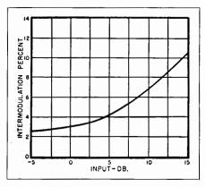
Fig. 3-18. Intermodulation distortion vs. recording level.
