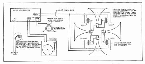
Fig. 22-15. A 75-100 watt church steeple installation. (Courtesy University)
