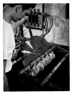
Fig. 27-6. The nickel plating operation which forms a protective surface.
