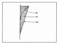
Fig. 7-16. Enlarged view showing comparatively large width of a standard (0.0005) single facet (S1) in contrast with the small aggregate widths of the dauble facets (1a and 1b), each of which is 0.001". Crass-hatched section shows amount of groove material that will be displaced by double-faceted stylus. This area plus shaded portion of the above stylus constitutes mass that will be displaced by single-faceted stylus. (Courtesy, F. L. Capps)
