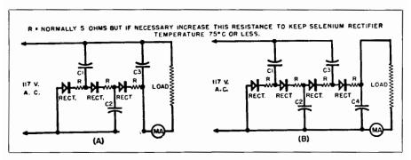
Fig. 19-29. (A) Voltage tripler circuit using three 200 ma. selenium rectifiers. With 40 mfd for C<sub>1</sub>, C<sub>2</sub>, and C<sub>3</sub>, a dc output of 325 volts can be obtained with a load of 200 ma. (B) Voltage quadrupler circuit using four 200 ma. selenium rectifiers. With 40 mfd for C<sub>1</sub>, C<sub>2</sub>, C<sub>3</sub>, and C<sub>4</sub>, a dc output of 425 volts can be abtained at 200 ma.
