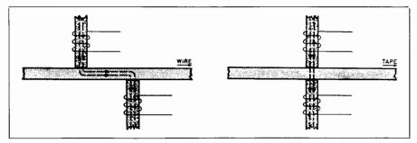
Fig. 11-3. (A) Longitudinol magnetization of wire using two pole pieces. (B) Perpendicular magnetization of tape using two pole pieces.
