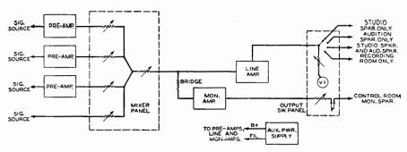
Fig. 26-29. Installation which provides for the use of three incoming audio lines.
