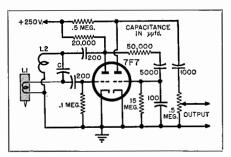
Fig. 9-13. Movement of pickup stylus amplitude-madulates an oscillating detector amplifier. Audio signal is obtained at output.
