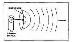
Fig. 1-3. Sound waves created by the movement of a mechanically-driven diaphrogm.
