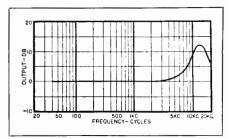
Fig. 3-15. Response of recording equalizer.
