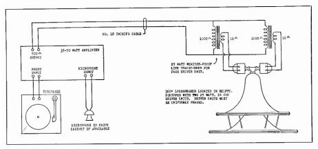
Fig. 22-14. A typical church steeple installation. (Courtesy University)
