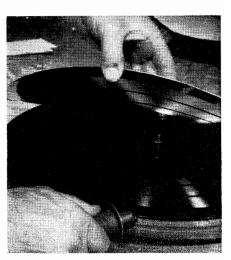
Fig. 27-4. Stripping the metal "master" fram the "master" recording.
