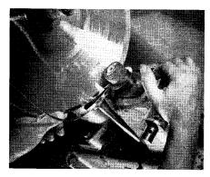
Fig. 27-12. "Stamper" is punched and sheared to fit die of the record press.
