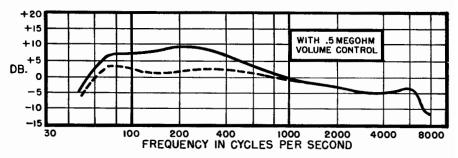
Fig. 4-13. Solid curve shows response of conventional crystal pickup when used without correcting filter. Dashed curve shows response using circuit of Fig. 4-14.
