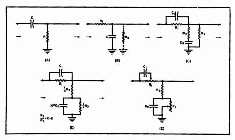
Fig. 16-8. Basic RC networks for frequency-response correction. (A) Low frequency attenuation. (B) High frequency attenuation. (C) and (D). Low ond high frequency lift. (E) Variable low and high frequency lift.
