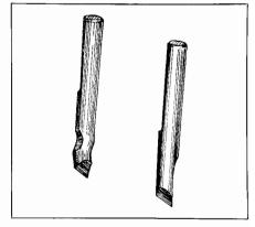
Fig. 5-2. Details of steel home recording styli.
