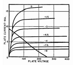
Fig. 19-41. Characteristic curves of 6SK7 with load line drawn as explained in the text. Numbers on curves are values of control grid bias.
