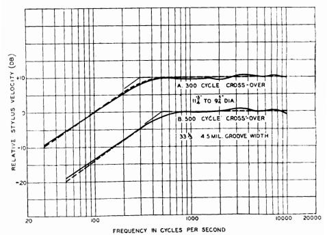
Fig. 5-34. Filter with additional network for 300 cycle crossover and comparison with the 500 cycle crossover adjustment.
