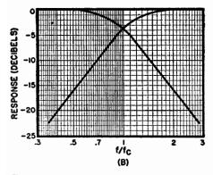
Fig. 16-16. Response curves of networks shown in Table 9. (A) is for the upper two networks, and (B) is for the lower two.
