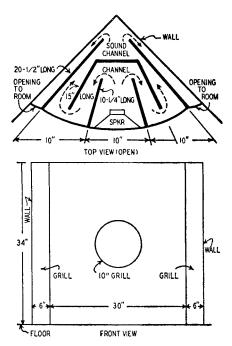
Fig. 15-3. Construction of a corner type enclosure for use with a folded exponential speaker.
