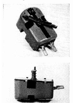
Fig. 9-34. Construction of the GE Model 12D triple play cartridge. (Courtesy, General Elect.)
