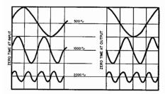
Fig. 28-14. Input and output phase relationships with theoretical linear phase shift of 0.18° per cycle. Note that time delay is constant at all frequencies—hence resultant wavefarm will not be changed.
