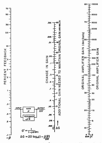
In negative feedback amplifier considerations  $\beta$  (expressed as a percentage) has a negative value. A line across  $\beta$  and  $\mu$  scales will intersect center scale to indicate change in gain resulting. It also indicates amount (in decibels) by which input must be increased to maintain original output. Original amplifications may be expressed as voltage ratio in decibels by using appropriate scale at right. (Courtesy Federal T&T Co.)
