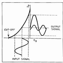
Fig. 28-1. Distortion in non-lineor amplifier.
