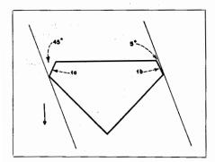
Fig. 7-11. Cross-section of same stylus in groove with 20° slope. Change in angular relationship between burnishing facets and groove is shown. Facet 1a forms angle of 45° with adjacent groove wall. Facet 1b on opposite side of stylus forms angle of 5° with its adjacent wall. In this and subsequent illustrations groove slopes in the opposite direction will merely reverse the effects described. (Courtesy, F. L. Capps)
