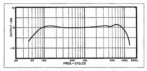
Fig. 3-17. Over-all frequency response of 35 mm. magnetic recording system.
