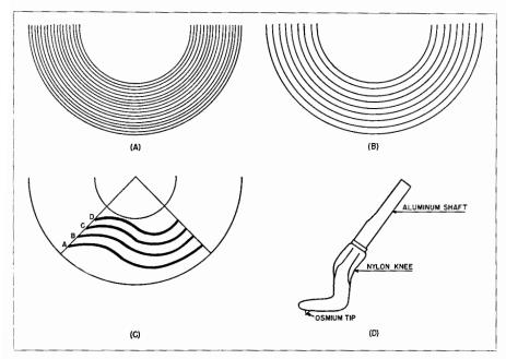
Fig. 6-1. (A ond B) Comparison of the number of grooves cut on a (A) Microgroove and (B) standard recording. (C) An exaggerated example of the "pinch effect." (D) The Webster-Chicago nylon "knee-action" needle designed to be used with Microgroove records.
