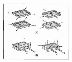
Fig. 4-26. (A) Single electrode plates in relative pre-assembled positions. Arrows show directions of maximum instantaneous strains for the indicated applied voltage palarity. (B) Arrows show location and direction of maximum motion of the element relative to the indicated axis.
