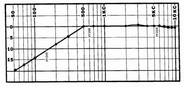
Fig. 28-42B. Frequency response curve of No. 2000S.
