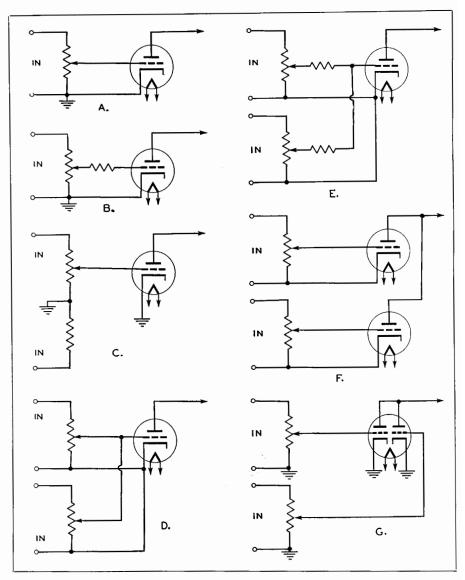
Fig. 18-1. High impedance circuits for general uses. Representative controls of the potentiometer variety.
