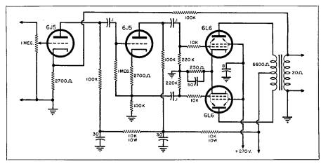
Fig. 19-35. The 6L6 push-pull amplifier of proven value and good design.
