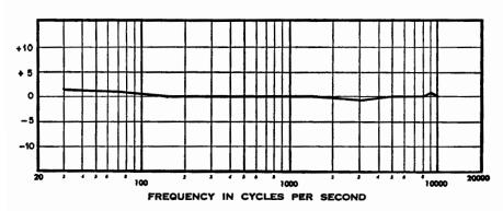
Fig. 9-31. Response curve of the Audax Polyphase cartridge based on constant stylus velocity.
