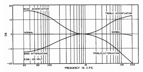
Fig. 24-13. Audio (tone control) characteristics.
