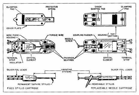
Fig. 9-2. Note the differences in construction between the fixed needle (left) and the replaceable needle (right) cortridge.
