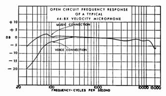
Fig. 14-12. Open circuit frequency response of RCA 44-BX velocity microphone.
