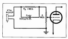
Fig. 4-14. Simple filter network that is often used for bass attenuation.
