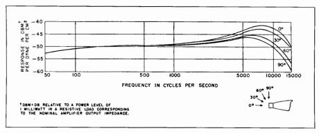
Fig. 14-24. Typical free-field response of 640AA condenser microphone in combination with RA 1095 amplifier.
