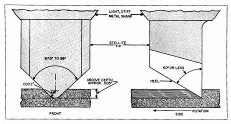
Fig. 7-4. Essential dimensions for steel or "Stellite" cutting stylus.
