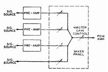
Fig. 26-28. Set up for multiple channel mixing.
