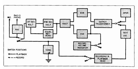
Fig. 12-1. Block diagram of a self-contained portable magnetic tape recorder.
