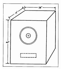
Fig. 15-37. Perspective view of a cabinet having the shape of a rectangular parallelepiped. The dimensions given yield the same volume as the cabinet shown in Fig. 15-32.
