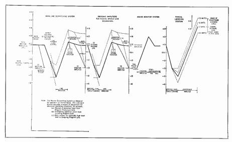
Fig. 25-2A. Typical level diagram of master dispatch systems and studio speech input equipment.
