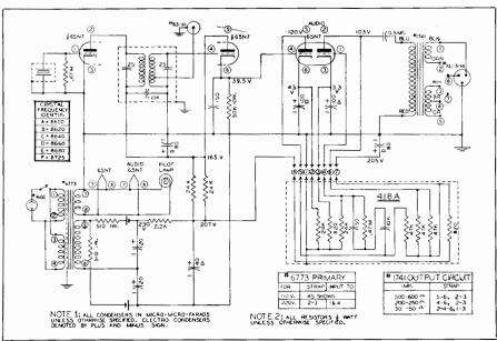
Fig. 14-33. Amplifier schematic of the OD-4C oscillator-demodulator for use with the Stephens C-2S microphone.
