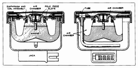
Fig. 14-8. Cross-section view of moving coil microphone.
