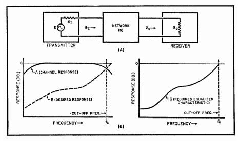
Fig. 16-6. (A) Generalized communication circuit including a 4-terminal network. (B) Frequency response curves showing required equalization to obtain desired response.
