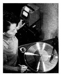
Fig. 27-9. Technician making sound test of the metal "mother" recording.
