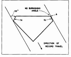
Fig. 7-12A. Same stylus cross-section in groove whose slope is 30°. Burnishing facet 1a forms angle of 55° with adjacent wall. Facet 1b cannot burnish with groove slope in excess of its basic angle. In fact, the edge formed by the meeting of cutting face and burnishing facet (A) will tear the adjacent graove wall. (Caurtesy, F. L. Capps)
