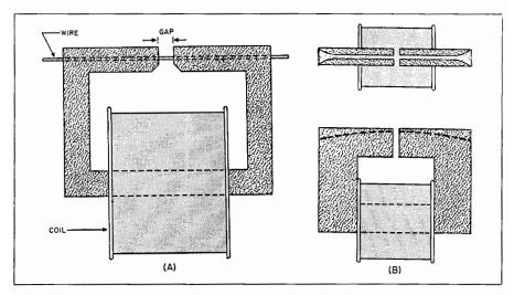
Fig. 11-10. (A) Typical wire record-reproduce head. (B) Open type wire record-reproduce head.
