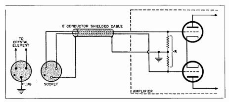
Fig. 14-5. Input connections for sound cell microphones.
