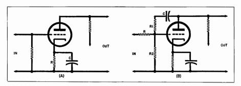
Fig. 17-5. (A) This circuit will boost the higher frequencies when condenser C is of toa low a value to provide an adequate bypass for the cathode resistor at the reference and lower frequencies. (B) By choosing component values, this circuit can provide inverse feedback on the highs.
