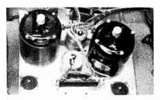
Fig. 5-16. Two hysteresis type motors rim-drive the turntable through rubber idler rollers.
