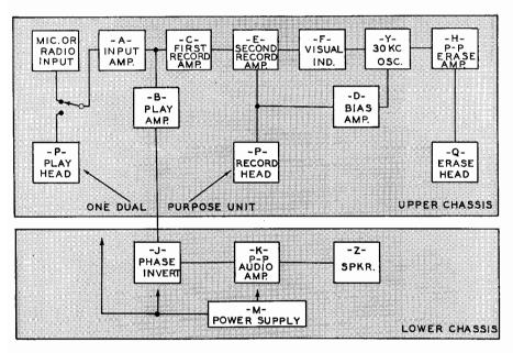
Fig. 12-15. Block diagram shows functional operation of tape recorder.
