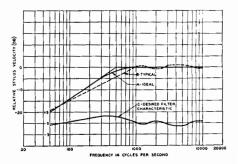
Fig. 5-28. Curves showing A (ideal cutter characteristic) B (typical response of MI-11850-C recarding head) C (difference between A and B which gives the desired filter characteristic).
