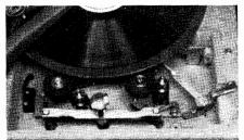
Fig. 5-19. Shows the position of the idlers with speed change knob "up" at 33 1/3 rpm.
