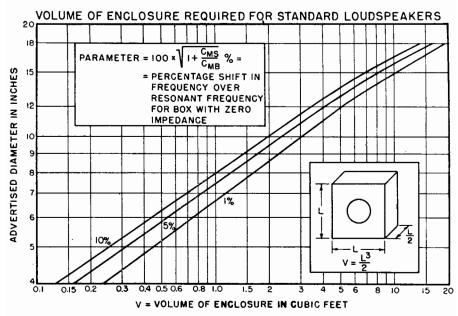
Fig. 15-14. Chart shows enclosure requirements, determined by means of formulae set forth in the text.
