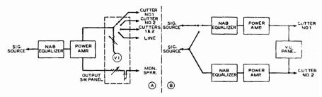
Fig. 26-25. Alternate arrangements for feeding two recorder channels.
