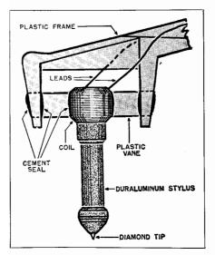
Fig. 9-21. The Fairchild dynamic pickup, Enlarged view shows assembly of unit.
