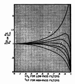
Fig. 16-11. Effect of porameter m on image impedance characteristics.
