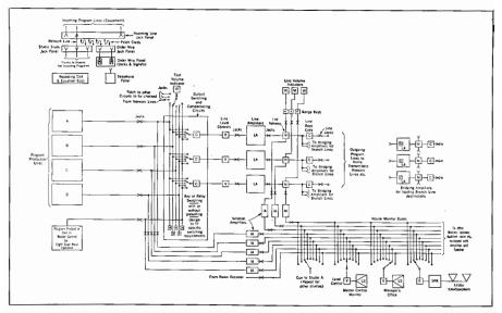
Fig. 25-2. Master dispatch systems showing types of facilities used. Quantities of inputs and other circuits will vary according to individual requirements. (Courtesy Western Electric)
