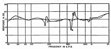
Fig. 15-34. Response frequency characteristics of a 15" loudspeaker mechanism mounted in the cabinet shown in Fig. 15-32. (A) Good response obtained by treating inside of cabinet with damping material.
