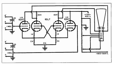
loscope as shown in Fig. 19-17. No change in the pattern on the cathode ray tube can be observed when the ground terminal of the cross coupled stage is connected to the center tap of transformer winding or to either input grid.
