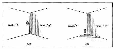
Fig. 15-1. (A) Speaker mounted adjacent to one side wall. Radiation into a solid angle increases low frequency efficiency. (B) Radiation into twa solid angles doubles the effect obtained in (A).
