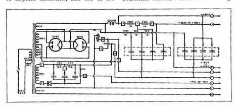
Fig. 21-2B. The power supply unit, including time delay relay, for use with the 50W-2 amplifier unit.
