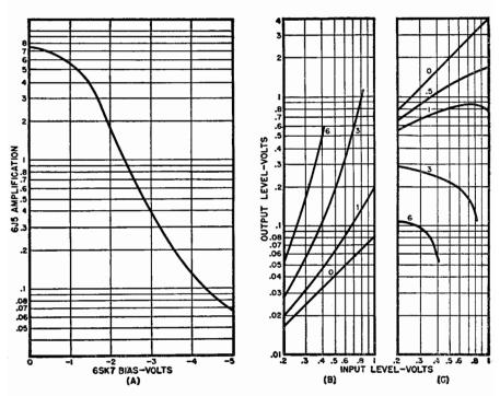
Fig. 19-42. (A) Relationship between the voltage amplification of the expander and the bias on the 65K7 control grid. (B) and (C) Performance curves for the circuit connected as an expander and compressor, respectively. The numbers on the curves denote the amplification of the signal fed to the 65K7 grid.
