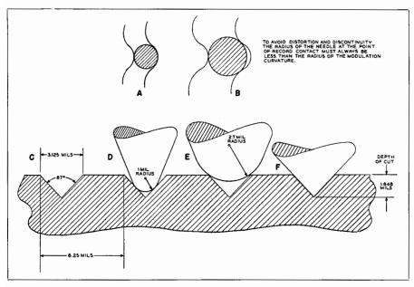
Fig. 5-3. Illustrating the action of groove fit of styli having various shapes.
