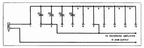
Fig. 4-20. Variable compensation for matching cutters and to nullify inductance.
