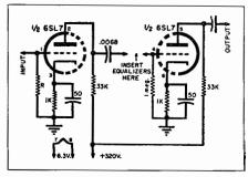
Fig. 20-1. Circuit diagram of preamplifier.
