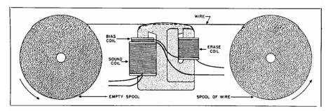
Fig. 3-20. Combined recard-playback head assembly for wire.
