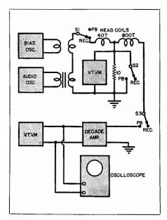
Fig. 12-6. Circuit diagram shows test setup for checking wave shape of bias oscillator.
