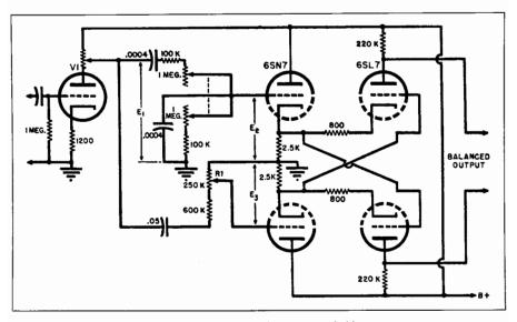
Fig. 19-19. Tone control circuit using cross coupled input stage.
