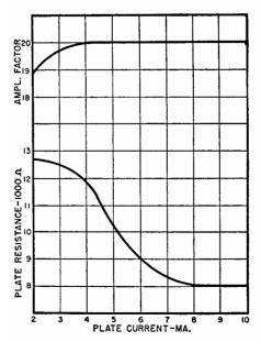
Fig. 19-45. Variation of amplification factor and plate resistance of the 6J5 with plate current, for circuit of Fig. 19-43.
