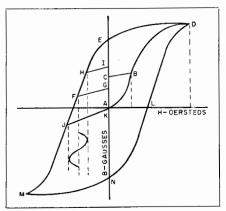
Fig. 11-7. Typical magnetic material magnetization characteristics.
