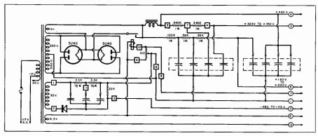
Fig. 26-21. Schematic of the McIntosh 50W-2 power supply showing protection relay circuit.
