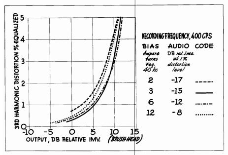
Fig. 11-20. Distortion as a Function of Output for Various Bias Currents. "Scotch" Sound Recording
