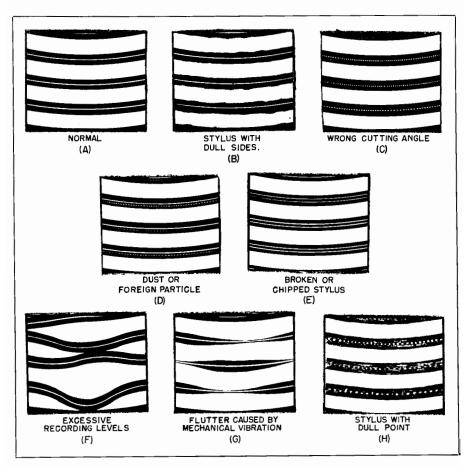
Fig. 7-7. Characteristics of recorded grooves. All except (F) have been cut without modulation.
