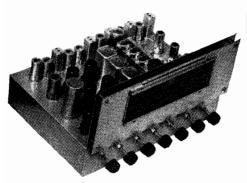
Fig. 24-7. The Collins 46-D FM-AM tuner. (Courtesy Collins Audio Products)
