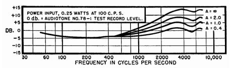
Fig. 4-16. Effect of resistance across cutter in pentode circuits. The ratio of the parollel resistance to the cutter impedance is represented by A.
