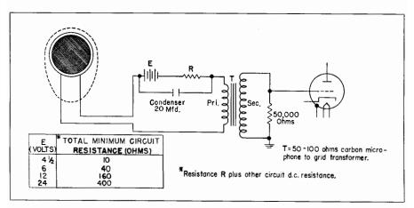
Fig. 14-3. Typical input circuit for carbon microphones of low impedance.
