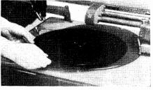
Fig. 5-21. Recording blank is here being placed in position and engages drive pin.
