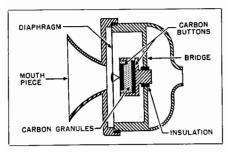
Fig. 14-1. Single button carbon microphone.
