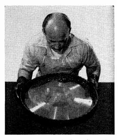
Fig. 27-1. Silverplating the "master" recording.
