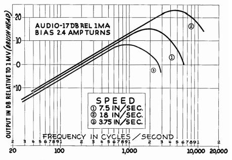
Fig. 11-19. Effect of Speed on Frequency Response. "Scotch" Sound Recording Tape No. 111.
