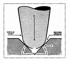
Fig. 9-7. Cross-sectional view of reproducing stylus in the record groove.
