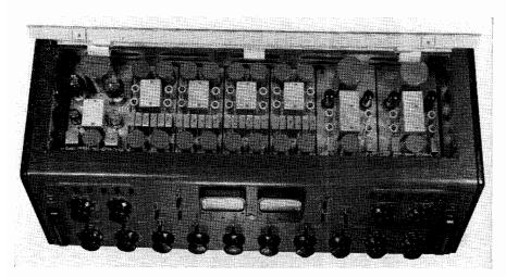
Fig. 25-3. The Collins 212A-1 speech input console for AM, TV and FM broadcast studios. (Courtesy Collins Radio Co.)
