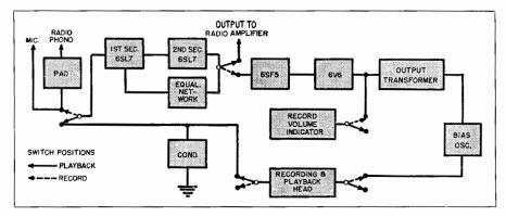
Fig. 12-2. Block diagram of radio adapter magnetic tape recorder.
