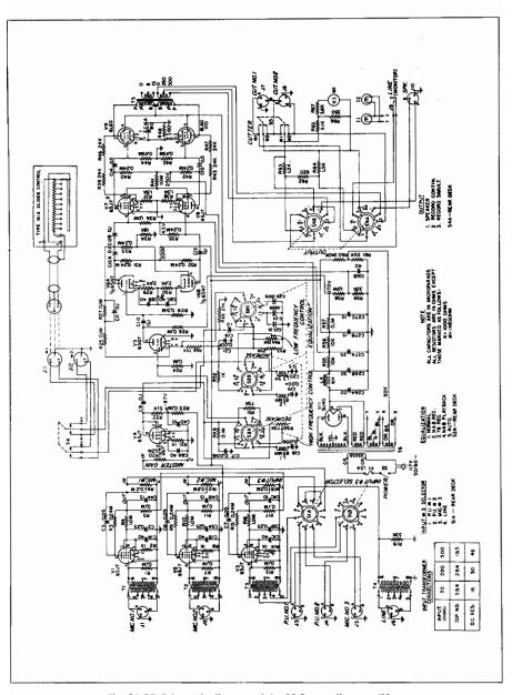
Fig. 26-35. Schematic diagram of the 90-B recording amplifier.
