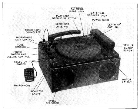
Fig. 5-1. The Meissner portable disc recorder, showing principal components and controls.
