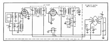
Fig. 24-3. Schematic of a two tube compact AM receiver as used in the Raytheon RC-1720 TV chassis.
