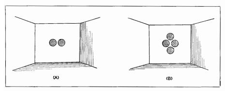
Fig. 15-2. Mounting speakers adjacent to each other increases low frequency response.
