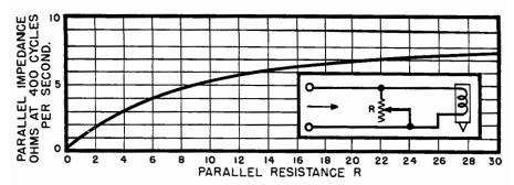
Fig. 4-17. Chart used to determine parallel 400 cycle impedance.
