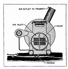
Fig. 2-5. Construction details of Parson's Auxetophone designed for intensifying sound by means of air pressure.
