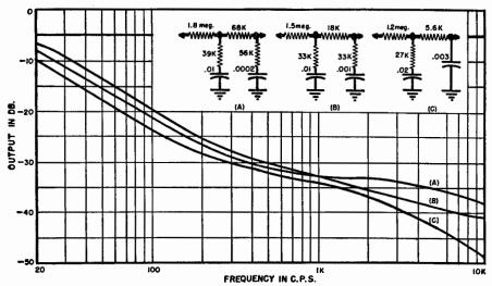
Fig. 20-4. (A) Equalizer and its response for Decca FFRR recards. (B) Frequency response and equalizer for Victor 78 rpm records. (C) Equalizer and response for Columbia 78 rpm records.
