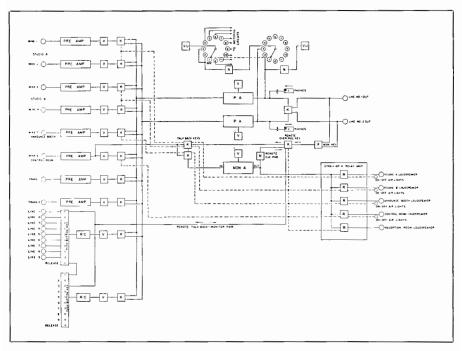
Fig. 25-5. Block diagram of the Collins 212A-1 speech input console. (Courtesy Collins Radio Co.)
