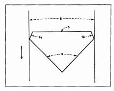
Fig. 7-10. Cross-section of standard lacquer recording stylus in unmodulated groove. Burnishing facets (1a and 1b) form 25° angles with groove walls (8). Arrow shows direction of record travel. Other facets: Cutting face (3) and clearance faces (4). (Courtesy, F. L. Capps)
