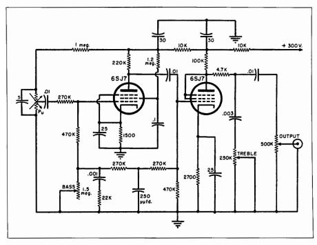
Fig. 20-14. Circuit diagram of the preamplifier.
