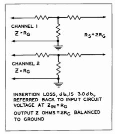
Fig. 18-7. The Two Channel series mixer.
