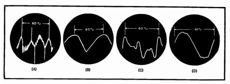
Fig. 28-34. (A) Noise pickup from fluorescent lamp. (B) Heater-cathode leakage current. (C) Inductive hum pickup by audio transformer. (D) Capacitive hum pickup from ac wiring.
