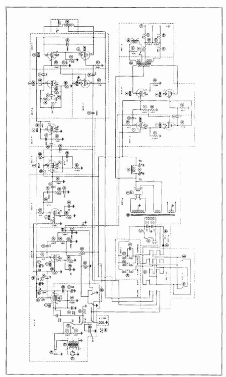
Fig. 12-14. Complete schematic diagram for "Soundmirror" tape recorder. A 30 kc. ultrasonic oscillator is used to demagnetize the tape.
