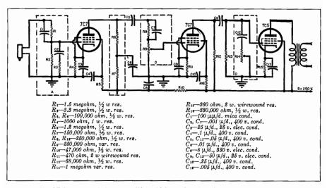
Fig. 17-6. A pentode input amplifier which provides bass boost action. See Table.
