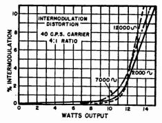
Fig. 21-5. Intermodulation distortion curves.
