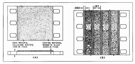
Fig. 3-13. (A) 35 mm. magnetic recording film. (B) Four-channel 35 mm. sound system.
