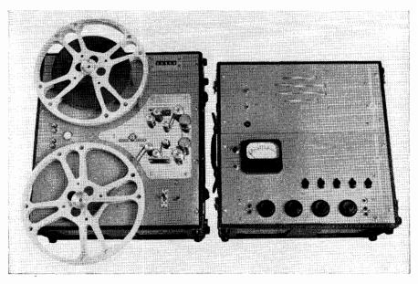
Fig. 13-11. The Stancil-Hoffman SR-Synchronous film recorder. (Courtesy Stancil-Hoffman)
