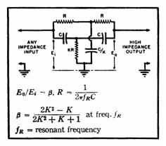
Fig. 16-20. Basic parallel—T R-C filter.
