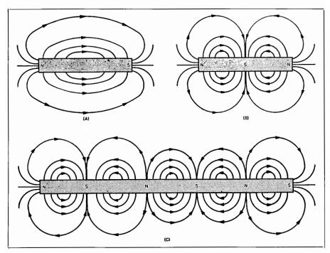
Fig. 11-1. Methods of magnetizing steel bars. (A) Dipole magnetized; (B) tripole magnetized; and (C) multipole magnetized steel bar.
