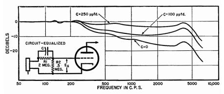
Fig. 9-4. Improved equalization is afforded by odding the RC circuit shown in the inset.
