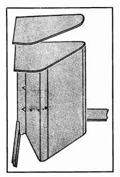
Fig. 15-11. Corner type cabinet, occupying only 15 cubic feet. Space above the cabinet is a mounting area for high-frequency horn.
