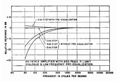
Fig. 13-7. Preamplifier gain-frequency characteristics.
