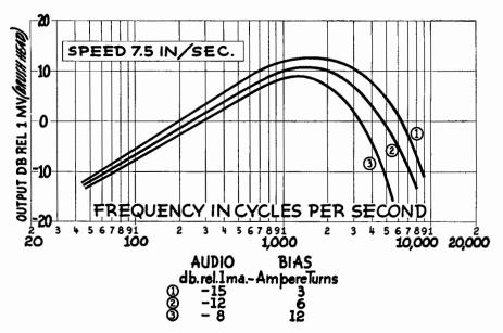
Fig 11-16. Effect of Bias an Frequency Response. "Scotch" Sound Recording Tape No. 100.
