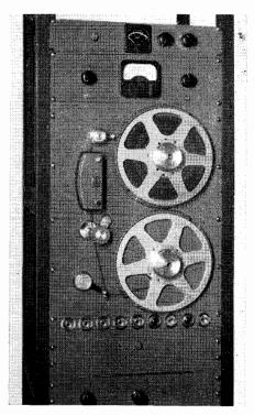
Fig. 12-23. The RCA Type RT-11A Magnetic Recorder. (Courtesy RCA)
