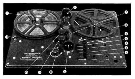
Fig. 12-16. Top view of Brush "Soundmirror" tope recorder. Keyed parts are; (1) Supply reel; (2) Reverse limit switch; (3) Brake shoe for head; (4) Takeup reel; (5) Forward push-bottom; (6) Reverse push-button; (7) Start push-button; (8) Stop push-button; (9) Record push-button; (10) Forward limit switch; (11) Drive capstan; (12) Record-reproduce head; (13) Erase head, and (14) On-off toggle switch.
