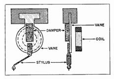
Fig. 9-12. Moving vane structure of Zenith "Cobra" pickup.
