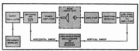
Fig. 23-4A. Measurement setup for determining reverberation time.
