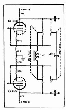
Fig. 17-21. Push-pull tone control circuit.
