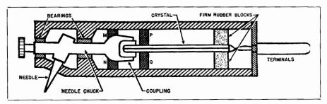
Fig. 9-6. Cross-section of construction details of typical cartridge employing rubber coupling between the needle and the chuck.
