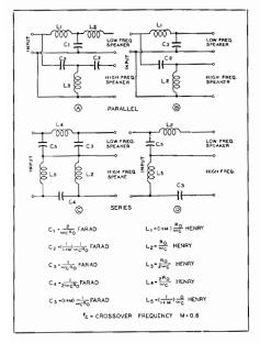
Fig. 16-2. Conventional series and parallel connected filter type networks along with the formulas for obtaining LC component values.
