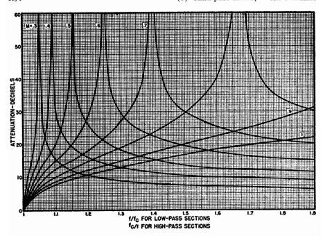
Fig. 16-10. Attenuation per section for low and high pass filters for various values of m.
