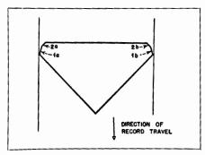
Fig. 7-17. Crass-section of an Anti-Noise Modulation Stylus having the leading facet 1a and 1b 0.0002" in width; and trailing facet 2a and 2b 0.0001" wide. (Courtesy, F. L. Capps)
