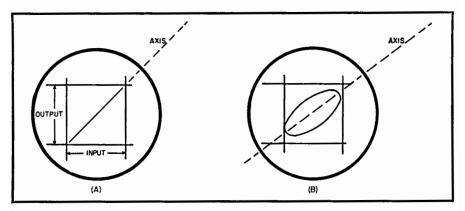
Fig. 28-12. Phase shift pattern—output vs. input. In (B) input is constant and output is attenuated.
