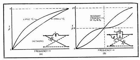
Fig. 16-14. Phase-shift characteristics of two simple types of all-pass sections.
