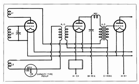
Fig. 2-11. How the capacity pickup of 1927 was connected to an audio amplifier.
