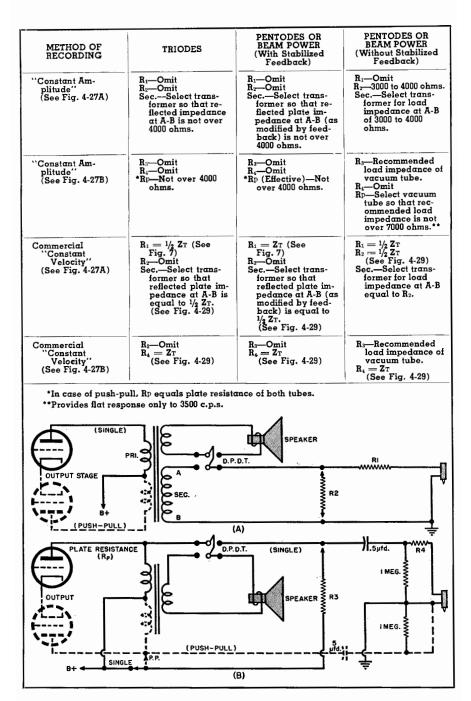
Fig. 4-27. (A) Schematic diagram shows cutter connected across transformer secondary. (B) Diagram shows how cutter may be connected directly across plates of output tube. Toble shown gives component values for either constant amplitude or constant velocity recording. Class "A" or "AB" single or push-pull output tubes should provide an undistorted power handling capacity of at least 3 watts.
