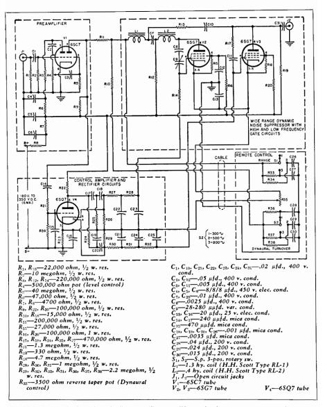
Fig. 20-9. Schematic shows how the "Dynaural" preomplifier and noise suppressor are combined in a single assembly. Connections for remote control are also indicated.
