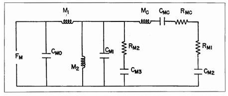
Fig. 9-23. Electrical circuit for a Bimorph phono cartridge.
