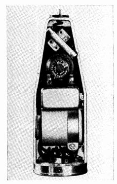
Fig. 14-25. The Western Electric RA-1095 amplifier. (Courtesy Western Electric)
