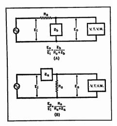
Fig. 16-7. Basic set-ups for experimental method of equalizer design.
