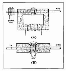
Fig. 11-4. (A) Cross-sectional view of magnetic wire recording head. (B) Drawing illustrates details of the recorder pole pieces.
