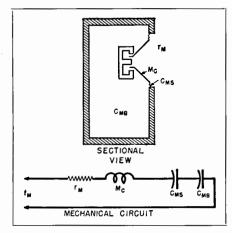
Fig. 15-30. Sectional view and mechanical circuit of a direct radiotor loudspeaker mechanism mounted in a completely enclosed cabinet. In the mechanical circuit  $F_m =$  driving force,  $r_m =$  mechanical resistance of air load and suspension system,  $M_c =$  mass of the cone, voice coil, and air load.  $C_{\rm MS} =$  compliance of the suspension system, and  $C_{\rm MB} =$  compliance due to the cabinet volume.
