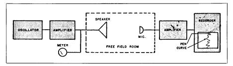
Fig. 15-28. Apparatus used to obtain response frequency characteristics of loudspeaker.
