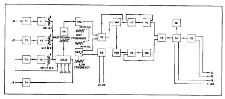
Fig. 26-34. Block diagram of the 90-B recording console.
