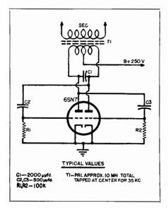
Fig. 12-7. Diagram of push-pull bias oscillator.
