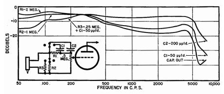
Fig. 9-5. High and low frequency response may be set independently with this equalizer.
