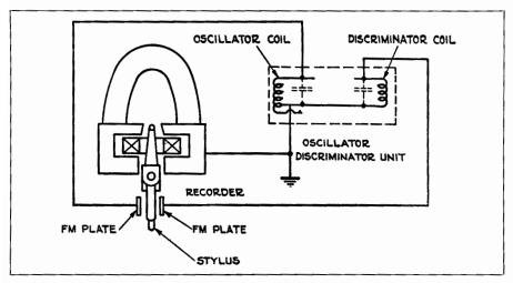
Fig. 28-44. Basic arrangement of the FM Calibrator. Small plates on either side of the stylus bar are connected to an oscillator discriminator unit mounted on the corrioge. (Courtesy RCA).
