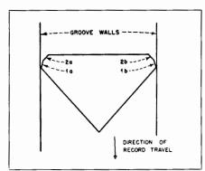
Fig. 7-13B. Cross-section of stylus shown in Fig. 7-13A in an unmodulated groove. The trailing facets 1a and 1b form burnishing angles of 15° with adjacent graove walls. (Caurtesy, F. L. Capps)
