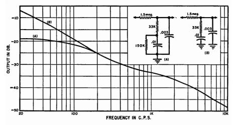
Fig. 20-3. (A) Equalizer for Columbia Microgroove recordings and its frequency response curve. (B)
