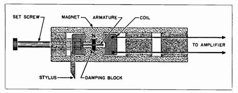
Fig. 4-12. Details of ossembly and structure of Shure Model 96 magnetic cutter.
