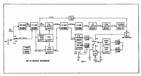
Fig. 24-9. Block diagrom showing switching arrangement employed in the Craftsman RC-10 tuner.
