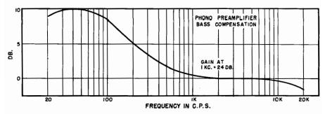
Fig. 24-12. Phono preamplifier characteristics.
