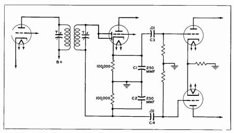
Fig. 19-15. Circuit diagram of a phase inverter which is somewhat unusual. Phase inversion takes place in the second detector stage of receiver.
