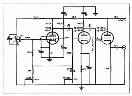
Fig. 9-11. The special preamplifier used with the strain-sensitive pickup. The cathode follower output permits the use of fairly long leads to a remote amplifier without excessive high frequency attenuation. High-impedance output may be taken from the plate of the first section of the dual triode if desired.
