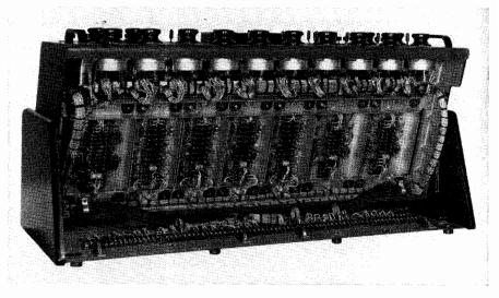
Fig. 25-4. Tilted or servicing position for the Collins speech input console. (Courtesy Collins Radio Co.)
