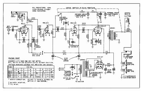
Fig. 5-1A. Schematic of electrical systems used in the Model 4DR disc recorder.
