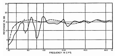
Fig. 15-33. Response frequency characteristic of a 15" loudspeaker mechanism mounted in a cabinet of the type shown in Fig. 15-32. (A) showing the elimination of deleterious effects due to the vibration of the cabinet by the use of heavy and well braced walls. (B) Response when deviations, i.e., walls made of thinner wood and the elimination of stiffeners, in the design of Fig. 15-32 were permitted.
