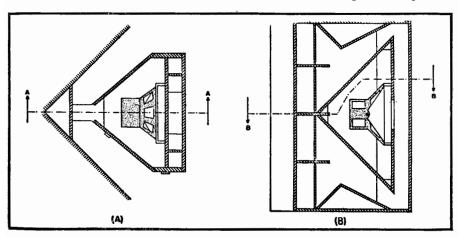
Fig. 15-10. The Klipschorn cabinet with 15" reproducer. Handles frequencies down to 30 cps, yet occupies only 15 cubic feet. Comparable theatre systems require 60 cubic feet or more.
