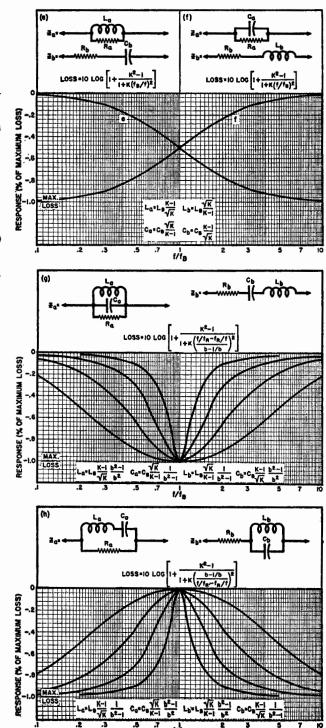
Table 2. Formulas and curves for equalizer design using several different networks for the  $Z_a$  and  $Z_b$  arms.
