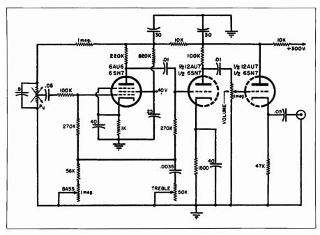
Fig. 20-18. Final circuit diagram of the improved preamplifier, model 2PRC-2.
