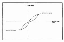
Fig. 11-15. Characteristic curve of a magnetic medium.
