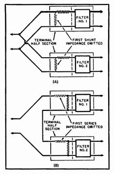
Fig. 16-13. Method of connecting complementary filters for operation in parallel and series.
