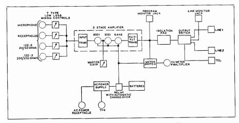
Fig. 25-7. Block diagram of the Collins 12Z remote amplifier.
