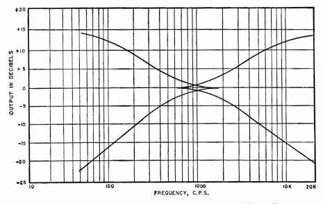
Fig. 17-24. Frequency response curves for the degenerative tone control discussed in text.
