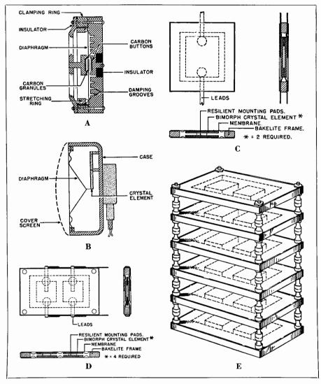
Fig. 14-4. (A) Double button carban, (B) crystal diaphragm, (C) single crystal element, (D) multiple crystal element and (E) six element sound cell construction.
