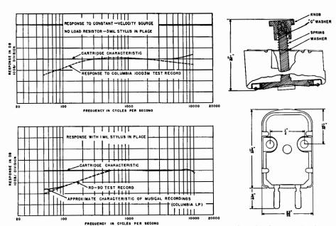
Fig. 9-35. Frequency response curves for both 1-mil and 3-mil styli of the Model 12D cartridge.
