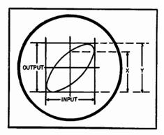
Fig. 28-15. Simple method of determining approximate phase shift by measurement of pattern— $\sin \phi = \chi/\gamma$ .
