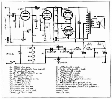
Fig. 19-27. Schematic diagram of 4-tube, 117 volt ac-dc audio amplifler.
