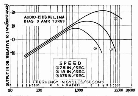
Fig. 11-18. Effect of Speed on Frequency Response. "Scotch" Sound Recording Tope No. 100.
