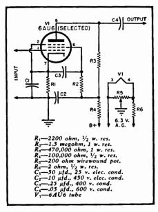
Fig. 28-31. Low-noise preamp using 6AU6.
