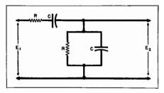
Fig. 19-20. RC network used in the above tone control circuit.
