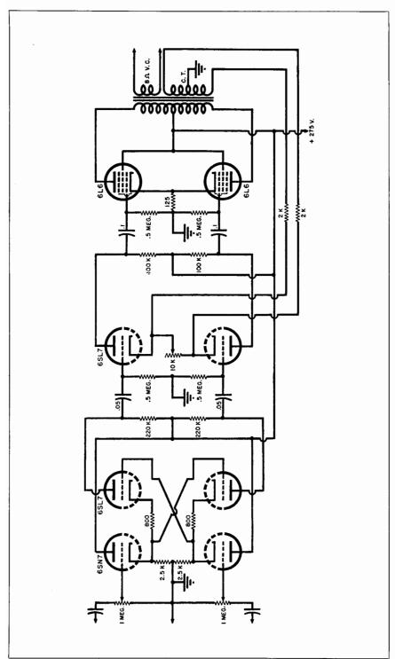
Fig. 19-21. Circuit diagram of a complete audio amplifler using a cross coupled input stage.
