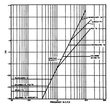
Fig. 20-16. Compensation required for matching best available estimates of current recording characteristics for ideal constant-amplitude type of transducer (asymptotes only).
