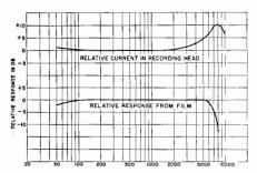
Fig. 13-10. 16-mm. frequency characteristics.
