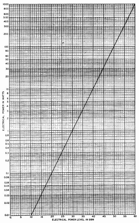
Fig. 22-4. Electrical power vs. electrical power level.
