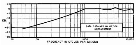
Fig. 4-19. Frequency response characteristics of cutter shown in Fig. 4-18.
