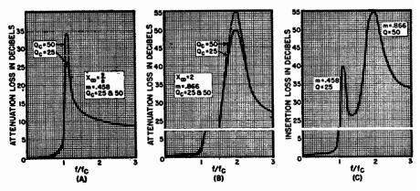
Fig. 16-21. (A) and (B) Attenuation curves of two different networks with different values of m, for two values of Q. (C) Attenuation characteristic of a composite filter made up of two of the sections shown in (A) and (B).
