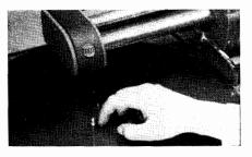
Fig. 5-20. Record drive pin comes up into position when this plunger-release button is pressed.
