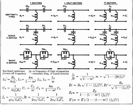
Table 6. Information for the design of high-pass filter sections.
