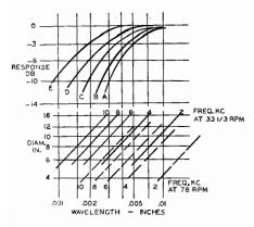
Fig. 7-28. Playback response vs. wavelength of recorded waves. The lower family of curves relates the wavelength to the frequencies ond diameter of records turning at 78 and 33 1/3 rpm.
