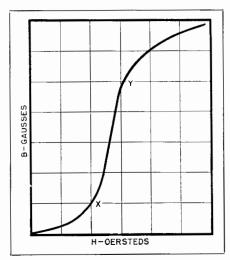
Fig. 11-8. Residual flux density curve.
