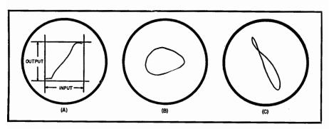
Fig. 28-13. Phase shift patterns—output vs. input. (A) Flat top distortion in output. (B) and (C) Various forms of non-linear distortion.
